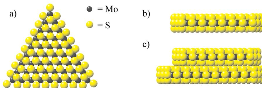
**Figure 2.** a) Atomic structure of a  $\text{MoS}_2$ -slab, showing the single Mo layer, sandwiched between two layers of S atoms. b) Side view of the slab, as it is visible in TEM measurements. c) A stack of slabs.
