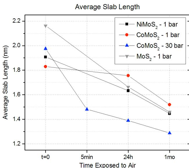
**Figure 3.** Average slab length as a function of exposure time to ambient air, showing a decrease in average length for all samples. Sulfidation pressures during sample preparation are indicated in the legend.
