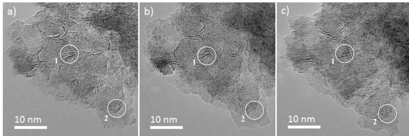
**Figure 1.** HRTEM images of  $\text{CoMoS}_2$  catalyst slabs on  $\gamma\text{-Al}_2\text{O}_3$  a) without any contact to air, b) the same sample region after 24 h of contact to air, c) the same sample region after 1 month in air. The sample region labeled '1' shows a stack of slabs that decreases in size after 24 h, while the sample region labeled '2' shows a slab that has completely disappeared after 24 h.
