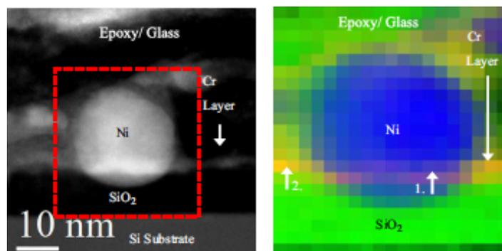
Fig. 2: High-angle annular dark field STEM image (left) of a Ni island supported by a roughly 10nm thick thermal  $\text{SiO}_2$  film. The right image shows the corresponding spectrum image with blue color representing Ni, red representing Cr, and green representing O. Reproduced with permission [3].
