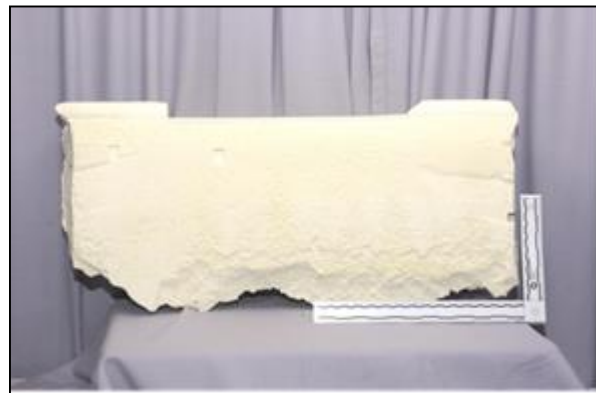
Figure 2. A two foot section of foam application that failed at less than 10 pounds per square inch (psig) pressure which for a normal application should have been 50 psig.
