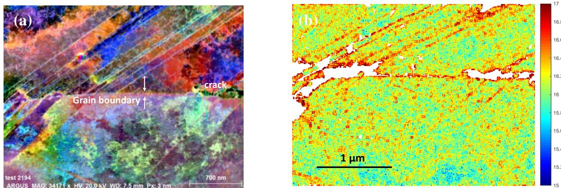
**Figure 1.** (a) FSE image showing the crack and the grain boundary (b) GND density map generated using 11 nm step size and the colour scale is dislocations per m<sup>2</sup> on a log<sub>10</sub> scale.
