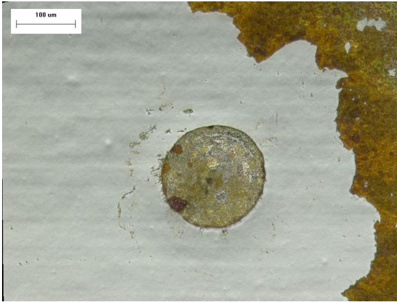
Figure 1 Digital Microscope image showing a circular defect with surrounding rust-coloured staining on a chrome plated surface.
