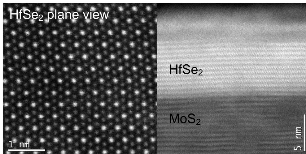
**Figure 1.** HAADF STEM of the (a) plane view and (b) cross section of 1T stacked HfSe<sub>2</sub> on MoS<sub>2</sub>
