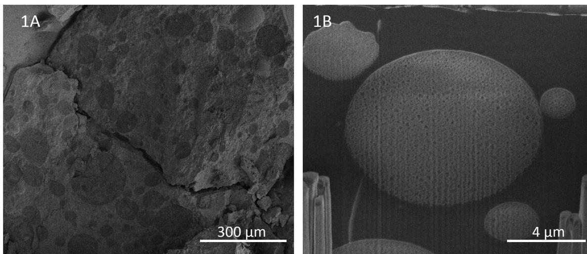
**Fig. 1:** CryoSEM images of emulsion droplets after freeze fracture (A) and FIB-milling (B) showing droplets ranging from 200 to 1 μm in diameters.
