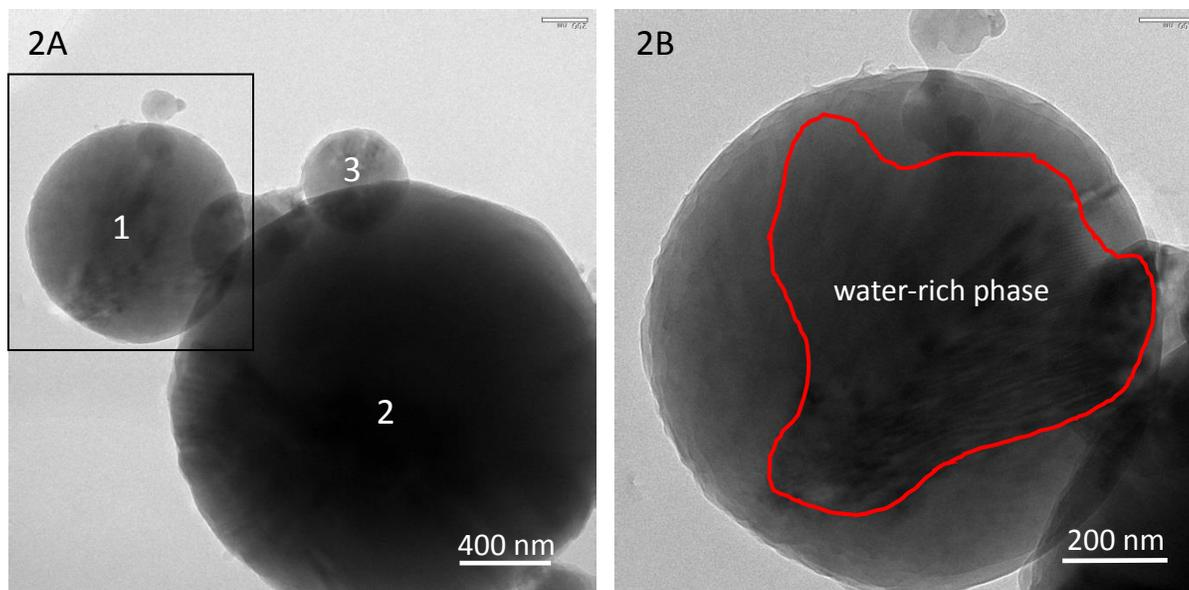
**Fig. 2:** CryoTEM images of emulsion droplets in bright-field-TEM mode using 300 keV energy electron beam. (A) Submicron size droplets (labeled as “1” and “3”) are suitable for TEM analysis. (B): A higher magnification of boxed area in A showing water-rich phase within the droplet (enclosed by “red” lines).
