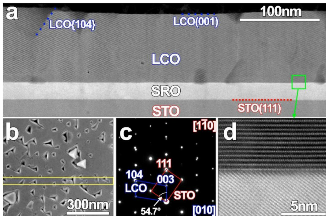
**Figure 1.** Characterization of the as-deposited LCO on STO(111) film by (a) STEM overview of cross-section, (b) SEM of a surface, (c) electron diffraction and (d) high resolution HAADF-STEM of LCO/SRO interface. The  $\{104\}$  planes are  $54.7^\circ$  with respect to the horizontal STO(111) cut plane.
