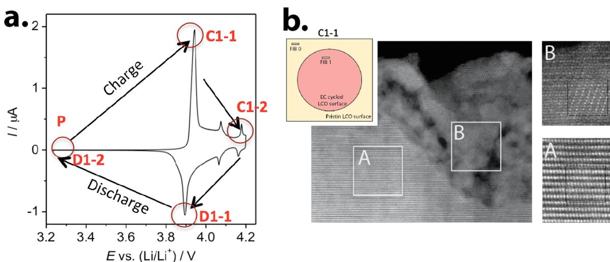
**Figure 2.** a. Cycling voltammogram of LCO/SRO/STO(111) film showing stages at which TEM samples were extracted; (b) Example of STEM imaging of a sample at C1-1 stage showing structural changes from layered (area A) to spinel-like (area B) structure in a near-surface region.
