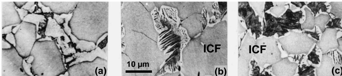
**Figure 1.** Intercritical ferrite (ICF) (grey) and epitaxial ferrite (white) revealed after cooling a 0.08C-1.47Mn-0.34Si-0.053Nb from a 4 min anneal at 810 °C, 12 °C/s (a), 135 °C/s (b), and 1000 °C/s (c); (etched with picral followed by alkaline chromate staining) [3].
