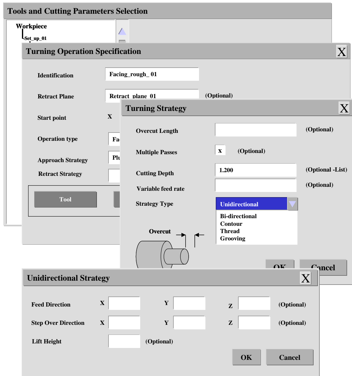
Figure 8.16 – The turning strategy dialog showing the cutting depth parameter
