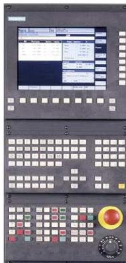
Figura 3.3: Interface Homem-Máquina.(ROMI 2008)
