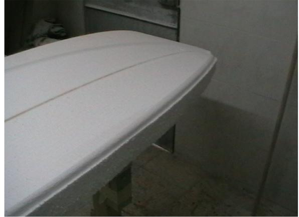
3. Place blank on machine supports with the deck facing up.
