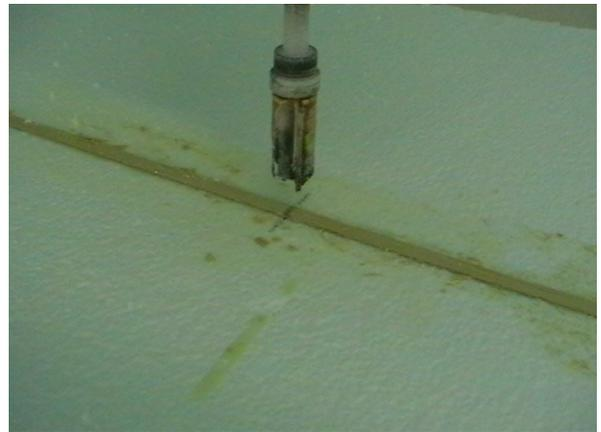
5. Lower the router by manually controlling the Z-axis in the Shapebot-program until the router bit sits a few mm over the blank (use a Feed override of around 20% to avoid hitting the blank with full speed).
