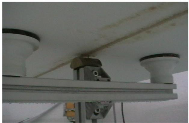
3. Adjust the position of the blank so that the mark aligns with the spikes on the left support and the stringer is centered between the spikes on both supports.
