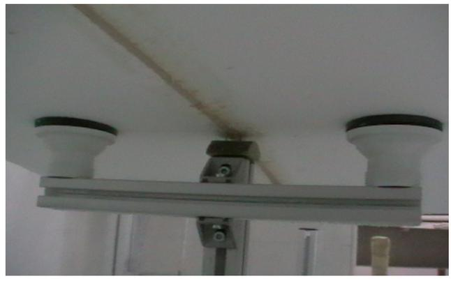
4. Lower the supports until the spikes enter fully into the blank.
