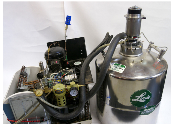
System overview showing a window air conditioner converted into a liquid cooler with liquid cooling lines running to the cryocooler which is mounted atop a Linde dewar. The additional refrigeration compressor mounted on top of the air conditioner unit compresses atmospheric air for liquid nitrogen production.
