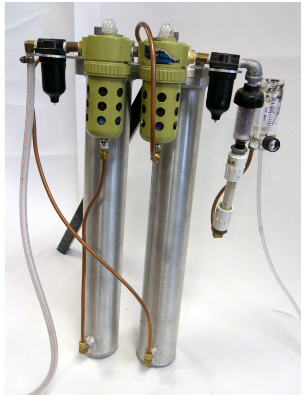
Air processing unit with two aluminum desiccator chambers, two small black coalescing filters, two beige carbon filters, nitrogen separation membrane at lower right, and a flow meter with needle valve.
