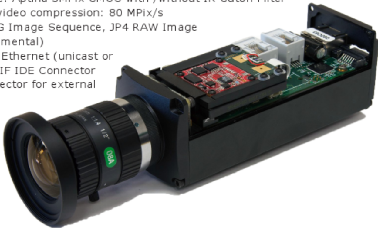
Elphel NC353L-369-GEO with lens, CF card and compass module (internally installed)
