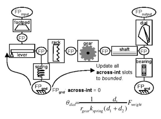
FP<sub>input</sub>: Through {[0 300]} Across-int {0} bounded Across Across-diff nil Class power Domain trans Interface feet Direction source FP<sub>output</sub>: Through bounded Across-int {[0 5]} bounded Across Across-diff nil Class power Domain rotate Interface dial Direction sink
