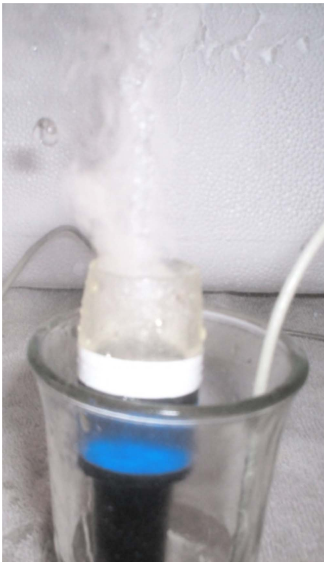
FIG. 7. (Color online) 1.54 MHz ultrasound transducer levitating and cavitating water at full system power.
