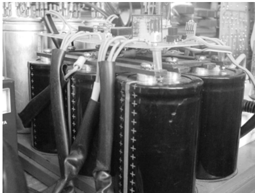
Fig 3b : Tank capacitor
