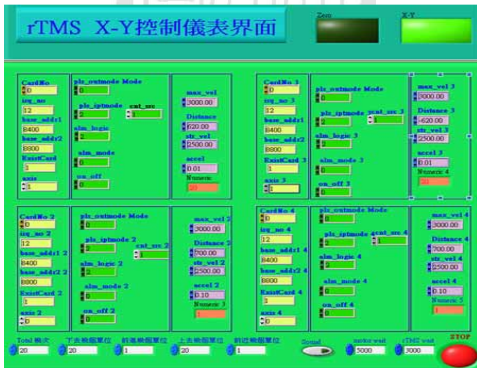
Figure 2.4. The graphical user interface developed in Labview for selecting the speed and position parameters.
