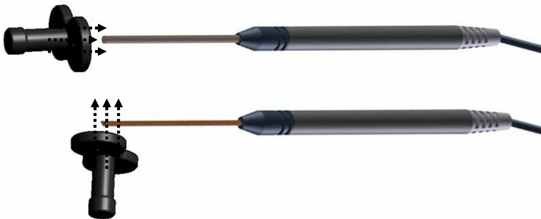
Figure 2.6. The use of (a) axial probe and (b) transverse probe for recording the magnetic flux in different orientations.
