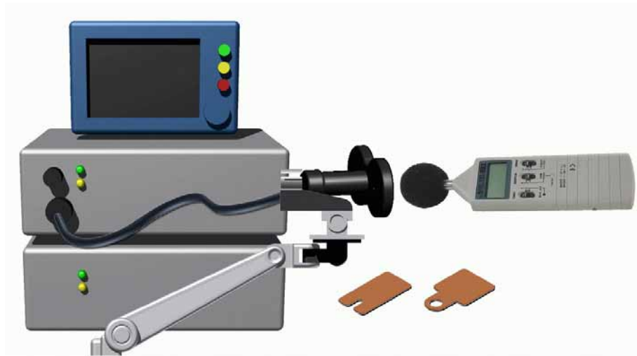
Figure 3.12. The use of digital sound level meter to measure the sound level for determining the threshold for ASR.
