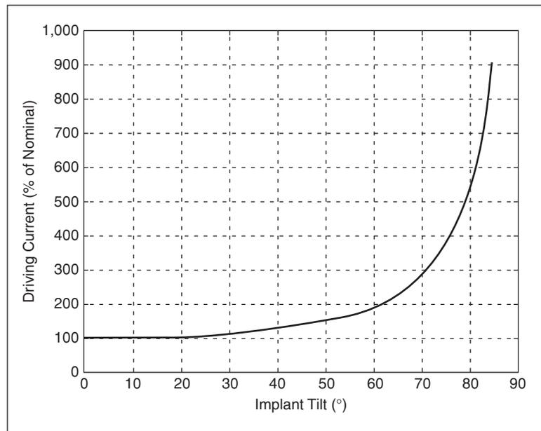
Fig. 6. The required nominal driving current versus implant tilt.
