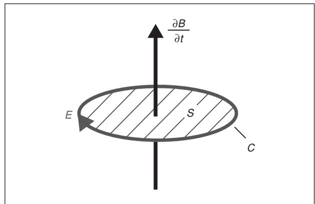
Fig. 2. Electric field induced in a conducting loop of  $n$  turns by a time-varying magnetic flux density.
