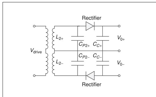
Fig. 5. The pickup coil circuit schematic.
