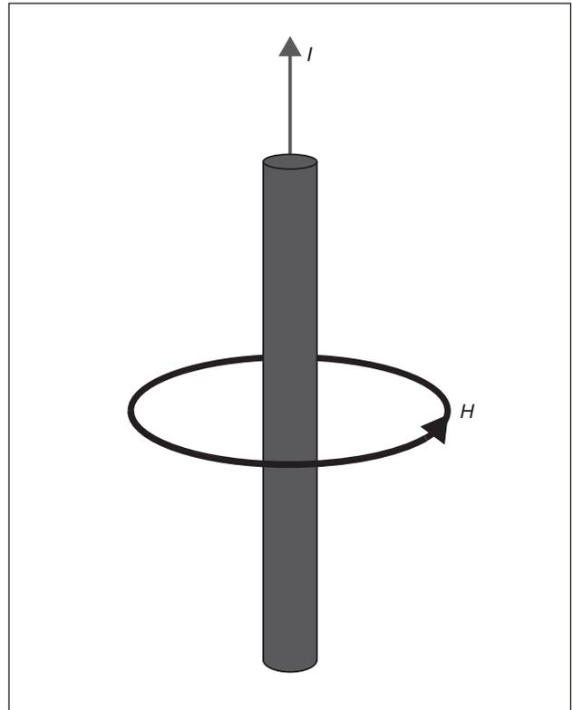
Fig. 1. Magnetic flux density surrounding a current-carrying conductor.
