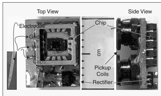
Fig. 9. Packaged transceiver photograph.
