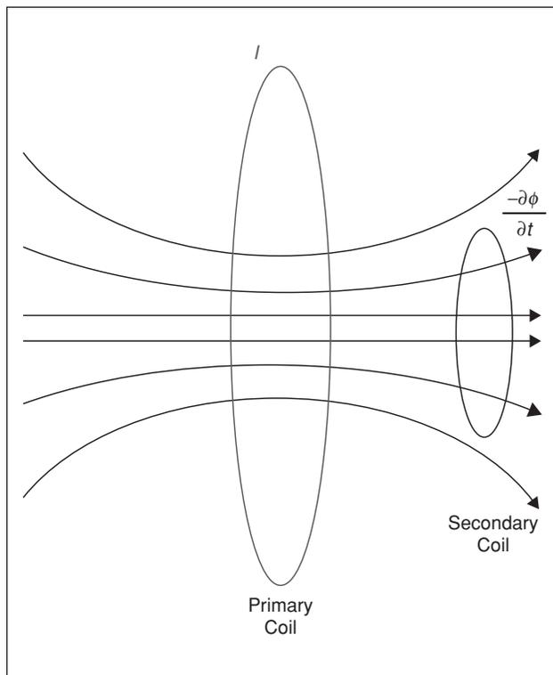
Fig. 3. A schematic illustration of the inductive powering process of a secondary coil by a primary coil.
