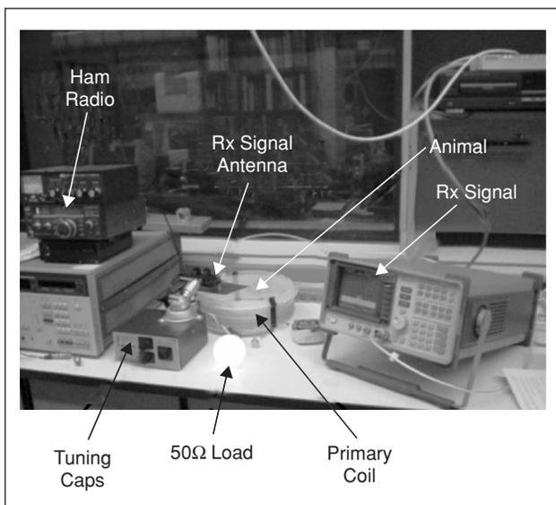
Fig. 8. A photograph of the complete inductive powering and RF telemetry setup photograph.
