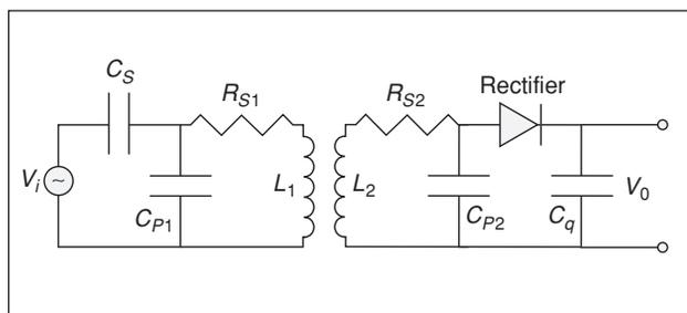
Fig. 4. The inductive power link schematic.
