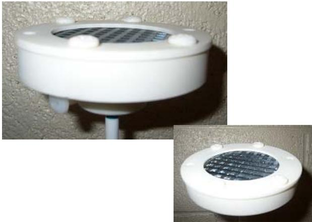
Figure 1: Picture of etching holder for wafer scale etching
