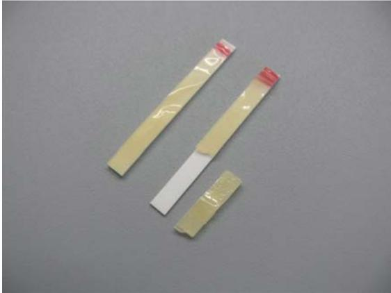
Figure 12: Loctite 5248 test sample beside peeled sample with cohesion break.
