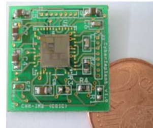
Fig. 5: Implant for sieve electrodes. The size is 20x20mm 2 . Die size 5.9x6.0 mm 2
