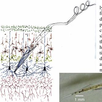
The basic format of the electrode lying within cortical tissue is shown in fig. 1. The six layers of cortex are diagrammed with the electrode tip in position near layer five that contains corticospinal tract cells. Neurites are shown growing into the tip, through the cone, and out the top end so as to hold the glass cone tip in position. The tip is introduced at an angle of 45 degrees from the surface of the cortex, and inserted for a distance of 5 to 6 mms until the part of the wire on the
