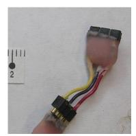
Finally, a removable handle is made by soldering larger diameter wires to a plug that inserts into the electrode connector. This allows for easy handling of the delicate electrode. The handle, shown here in fig.2.3.2f as three colored wires plugged into the electrode's connector, is itself connected to plugs in a sealed container box. The container allows safe storage and transport prior to implantation. Scale to the left of figure is in mms.
