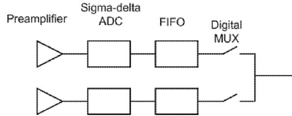
Figure 7. 1 ADC per channel architecture
