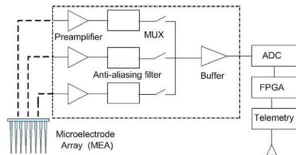
Figure 1. System architecture with off-chip ADC
