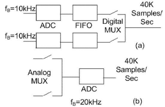
Figure 6. (a) 1 ADC per channel. (b) 1 ADC multiple channel.
