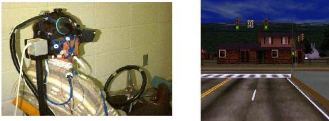
**Figure 5-1: (Left) An individual demonstrates driving in the modified go cart while wearing an electrode cap and head-mounted display. (Right) A typical stoplight scene in the virtual environment.**
