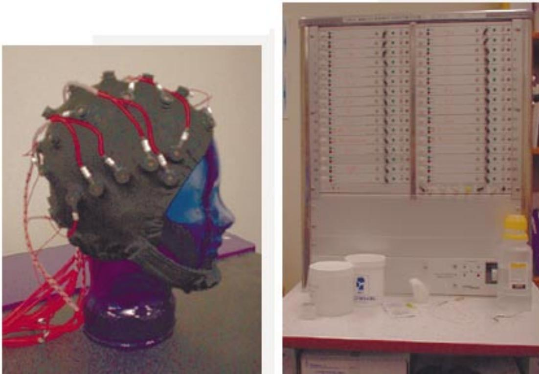
**Figure 1-1: (Left) A 32-channel electrode cap made by Neuromedical Supplies. (Right) A 32-channel set of analog Grass amplifiers.**
