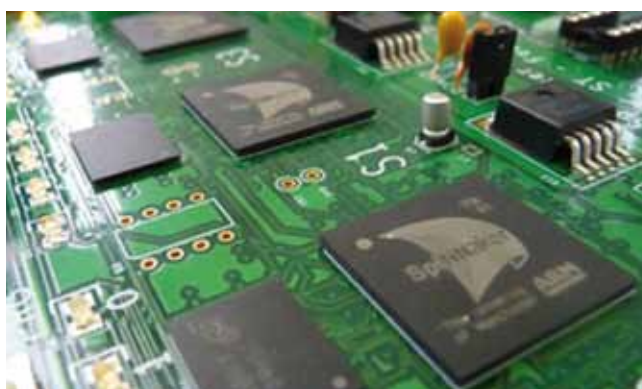
Figure 7: Precursor project: ARM-based, many-core chips from the SpiN-Naker project, Manchester University, United Kingdom
