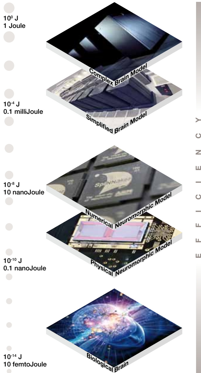
Figure 15: From biological brains to supercomputer simulations. Energy per synaptic transmission spans fourteen orders of magnitude. Neuromorphic computing occupies an intermediate position between biological brains and supercomputer simulations
