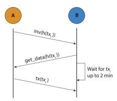
Fig. 1: Three-step protocol used to forward transactions in Bitcoin.
